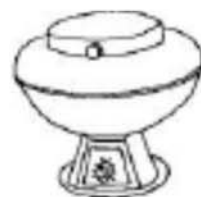
Centrifuge. Decant Supernate. Wash ppt with \text{H}_2\text{O} . Centrifuge. Decant.
