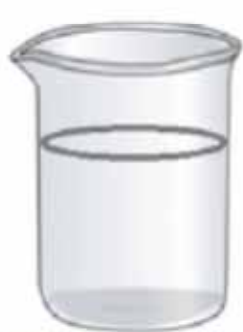
Water Sample in glass beaker. Acidify pH 2.
