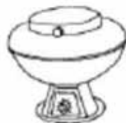
Centrifuge. Decant Supernate. Wash ppt with H 2 O. Centrifuge. Decant.
