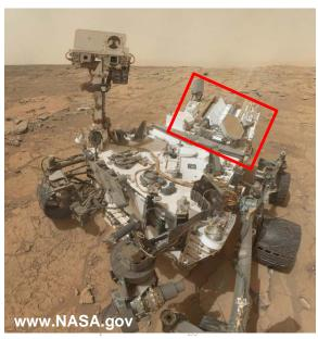
Mars Science Laboratory Curiosity: 8 general-purpose heat source modules, <u>4.8 kg</u> of PuO<sub>2</sub>
