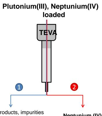
Fission Products, impurities in the (I),(II), and (III) Oxidation state and Pu(III) removed in 8N HCI + 5mM Hydroquinone
