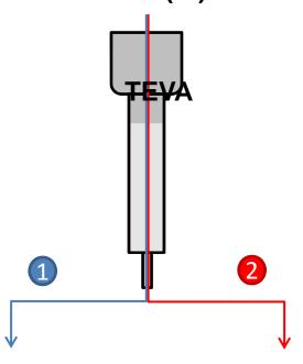
Fission Products, impurities in the (I),(II), and (III) Oxidation state and Np(V) removed in 4N HNO<sub>3</sub>
