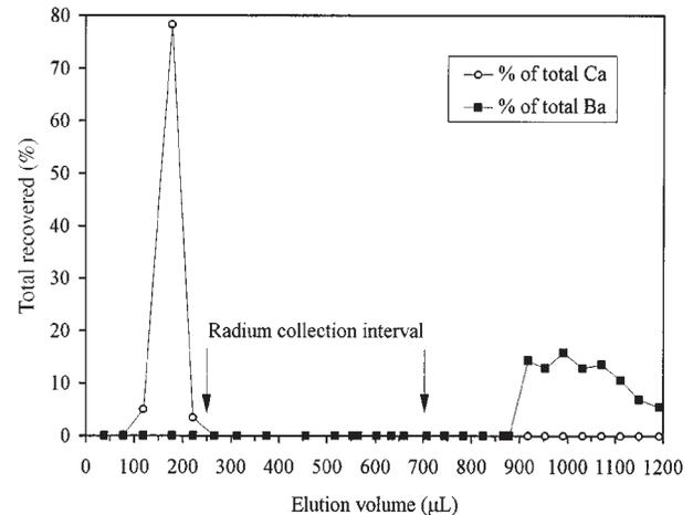
An acid strength of 1.1 N HNO<sub>3</sub> achieved the greatest separation between calcium, barium, and radium on the Sr<sup>®</sup> resin microcolumn. Based on the distribution coefficients of the Sr<sup>®</sup> resin, a radium sample collection interval of 250 to 700 μL was selected between the calcium and barium elution intervals (Fig. 4). A small sample spot (<0.5 mm) remained after drying and was used for radium determination on the TIMS.
