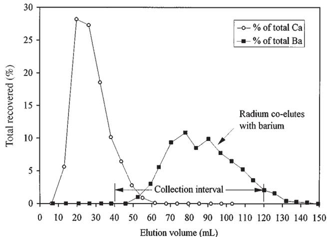
**Fig. 3.** Elution characteristics of the second pass using 6.0 N HCl on the AG<sup>®</sup> 50-X8 cation exchange column for calcium (○) and barium (■). To more clearly evaluate the separation, calcium and barium elutions were performed separately but were plotted together. The collection interval for the radium and barium fraction was from 40 to 120 mL
