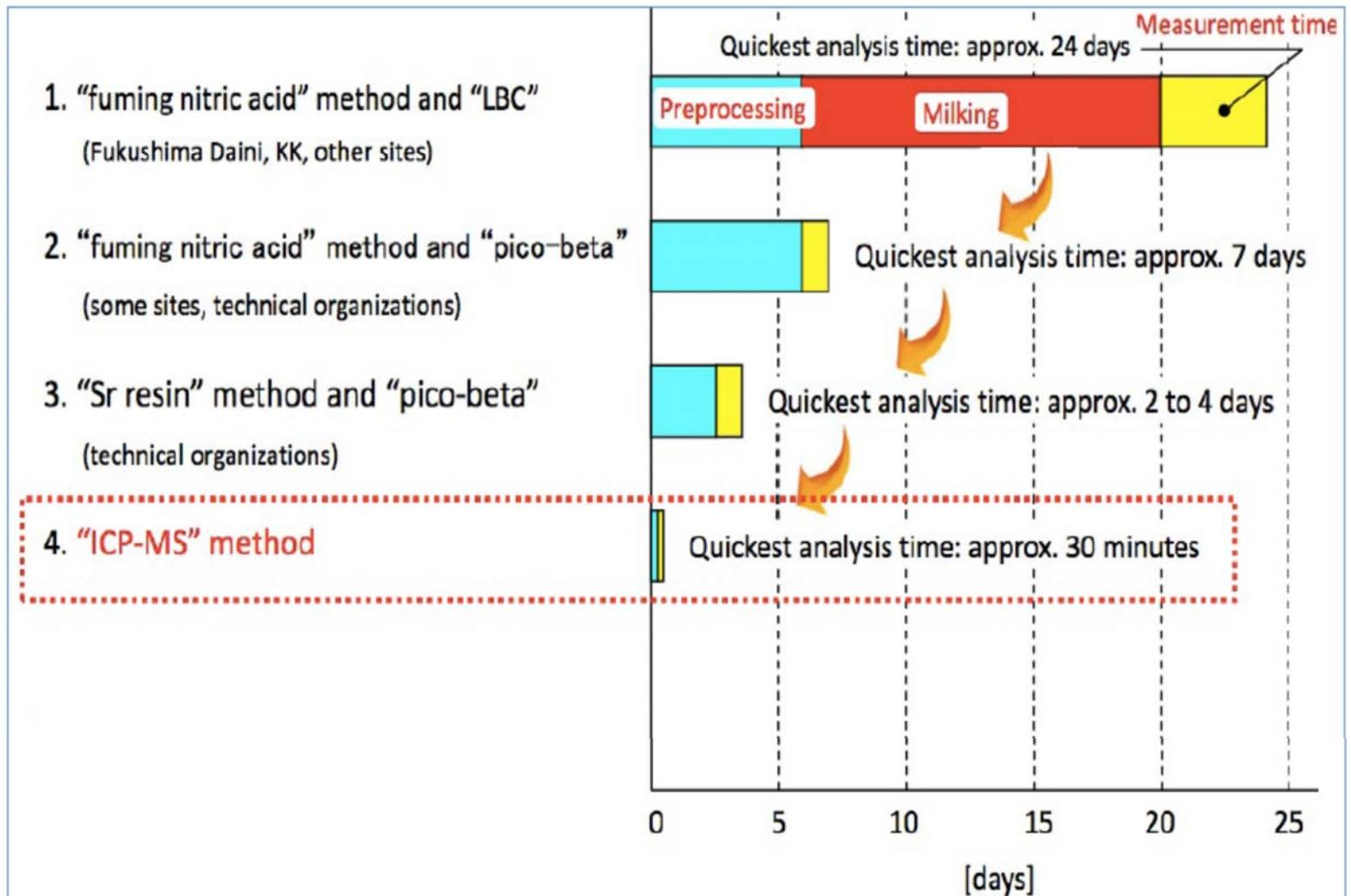
INNOVATIVE TECHNOLOGY TO PROVIDE FASTER RESULTS ON WATER QUALITY AT FUKUSHIMA
