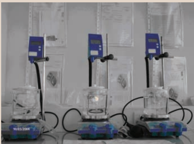
Figure 4 : Po-210 Auto-deposition unit.
