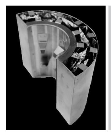
Shielded mirror reflective insulation is intended for permanent application on pipes that are both hot in temperature and radiologically. An inner layer of shielding made from T-Flex®, solid lead, or stainless steel is added to Trancso insulation. The amount of shielding is dependent on the amount of weight that can be added to the pipe. Two clamshell halves wrap around the pipe and are buckled together.
