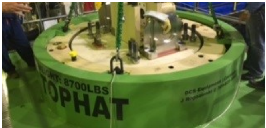
Clinton - Holtec Shield Bell with integrated work platform. Platform can be stood on and provides gamma and neutron reduction.
