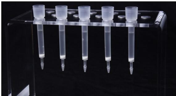
Add enough top frits for each column to a centrifuge tube with a small volume of 0.05M HNO<sub>3</sub>. Soak the frits to remove air bubbles. Swirl or vortex to mix, but avoid vigorous shaking.
