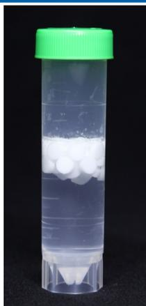
Decant the 0.05M HNO<sub>3</sub> from the empty columns. Mix the slurry of resin and 0.05M HNO<sub>3</sub> to suspend the resin. Add the resin slurry to each column until the reservoir above the column is ~half full. Allow the resin to settle (~1 hr).
