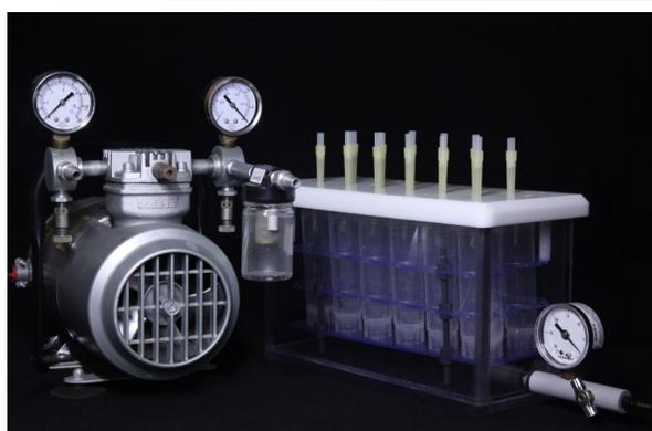
1) Obtain a 12-Hole or 24-Hole vacuum box, vacuum pump and tubing.
