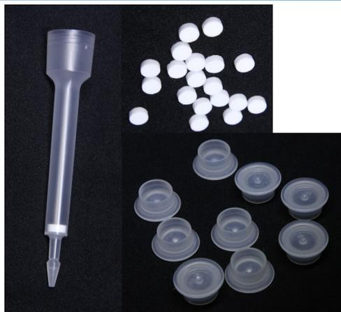
Eichrom snap tip 2 mL Columns (AC-141-AL) come with the bottom frit inserted. Top frits and column top caps are also included.
