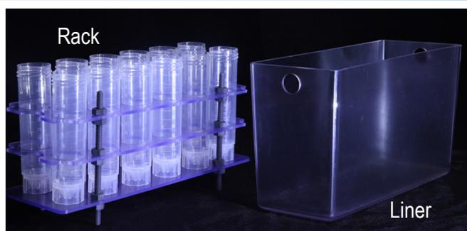
5) Sample aliquots may be collected in individual 50 mL centrifuge tubes or collectively in the vacuum box liner.
