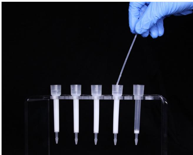
Full 2 mL columns should have a bed height of  $4.1 \pm 0.2$  cm. Add additional slurry to meet this height or remove excess resin using a plastic transfer pipet. Leave enough 0.05M HNO<sub>3</sub> above the packed bed to fill the column and a portion of the reservoir.
