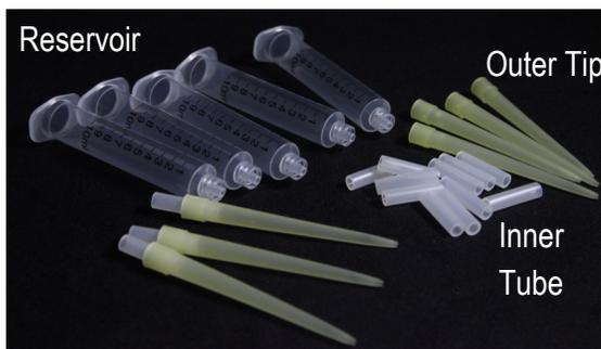
6) Change cartridge reservoirs and inner and outer tips prior to elution of each analyte to improve purity.
